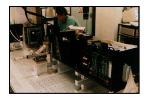
The above photographs show the Essex polarimeter with the calibration set-up for measuring the polarimeter transfer matrix.
