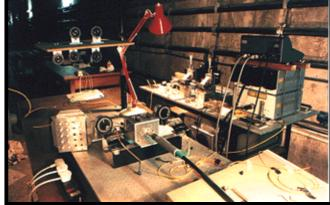
In the left picture, John's POTDR from the top. This time you can see the polarisation analysing box sitting above the four channel digitising oscilloscope. Finally we also used John's POTDR in the tunnel as you can see in the right picture.
